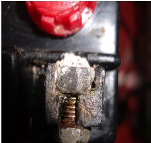
If you don't clean them completely, the corrosion will reappear soon. Coat the terminals with Vaseline or light grease to deter corrosion.
