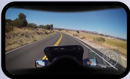
Similar in size to a slim GPS unit, the weatherproof NUVIZ uses a liquid-crystal on silicon (LCoS) microdisplay-based engine to project images onto a transparent combiner (a miniature windshield) mounted on the top of the unit, and is what the wearer actually looks through to see the projection. The screen will appear in the lower corner of the helmet eyeport. As with other HUDs, the image "focused" at infinity so the rider doesn't need to refocus from the road to view information.
