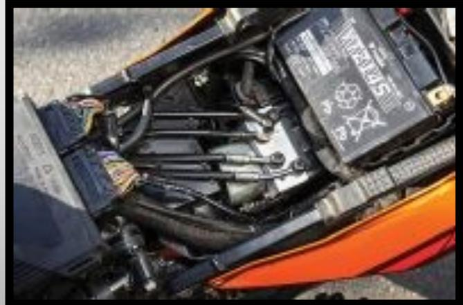
The key to never crashing on the brakes again? It's all right here under the seat, where the Bosch 9M ABS control module is located on the KTM 1190 Adventure.
