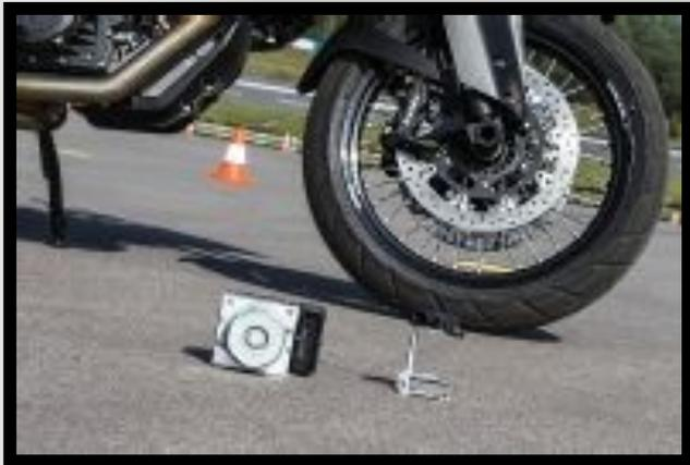
A control module (left) and lean-angle sensor (right) combine forces to create Bosch's Motorcycle Stability Control (MSC), the first ABS system informed by lean angle.
