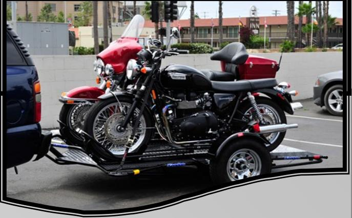
Tongue weight should be between 9% and 15% of the gross trailer weight fully loaded. Tongue weight is the weight of the trailer on the ball of the hitch, and can be measured with a bathroom scale under the trailer jack stand...close enough for gov't work...lol . Tongue weight towards 15%, generally provides a more stable tow with less sway than tongue weight less than 9%...
