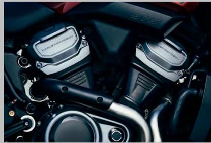
Minimizing weight and maximizing performance, the Revolution Max provides a narrow powertrain profile that is integrated into the motorcycle as a stressed member of the frame to enhance center of
