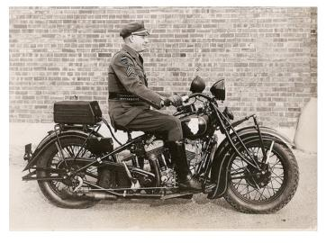
20 April 1936 ~ 300 motorcycles and 200 hundred autos of the Illinois State Highway Police are being equipped with radio receiving sets and transmitting stations, each with a range of about 70 miles, are being erected throughout the state. The above photo shows the receiver on the rear carrier of the motorcycle; a loud speaker is on the handlebars, facing he driver behind the headlight
