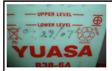
Do not overfill your battery. The heat will cause the electrolyte to boil over. You then have battery acid all over your engine or transmission cases. Wash it off immediately with a mixture of baking soda and water.
