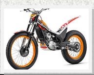
Montesa Honda Cota 4RT Repsol Edition (\$8,999): Coming in May, the limitededition Cota 4RT Repsol Edition is a Montesa trials bike powered by a Honda 260cc engine. The bike has fuel injection and a decompression system reducing engine braking, making the four-stroke motor perform like a two-stroke. Showa suspension and wide footpegs are notable features.
