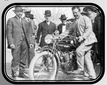
At that time, Harley-Davidson was producing the J-series motorcycle which were powered by a 61 cubic inch F-head engine and capable of speeds up to 60 miles per hour. The US Army ordered these in a variety of configurations including standard motorcycles for troop transport, sidecar equipped motorcycles for command transport, sidecar equipped motorcycles with machine guns and sidecar equipped motorcycles to carry supplies and ammunition.
