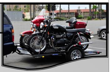
Tongue weight should be between 9% and 15% of the gross trailer weight fully loaded. Tongue weight is the weight of the trailer on the ball of the hitch, and can be measured with a bathroom scale under the trailer jack stand...close enough for gov't work...lol . weight towards 15%, generally provides a more stable tow with less sway than tongue weight less than 9%...
