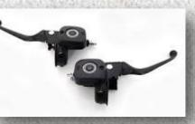
recalled because a component in the clutch master cylinder may fail, reducing the pressure available to keep the clutch disengaged.
