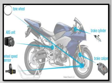
full force to the An antilock braking system works by constantly pedal/ measuring wheel speed. One common way to do this without is with a small grooved ring near the brake disc often fear of going in called a tone wheel. The wheel speed sensor sends the to a skid, but tone wheel readings to the ABS unit, which can deterthey still need to practice safe braking techniques and mine whether the wheel is about to stop rotating. If it
