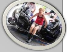
**#3 R**: Leaning the bike on the kick stand provides a lower left side for easier access, assures that the bike is stopped and, gives you a more stable platform for the CR to get on / off.
