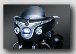
incorrect headlight was installed. The light output from the incorrect headlight can affect the motorcycle's visibility, increasing the risk of a crash.
