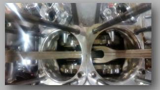
A new, or rebuilt, engine's cylinder bore may look smooth, but it can still be somewhat rough from the machining at the factory and the piston rings need time to create a good seal. This is needed to keep the combustion gases separate from the engine oil. If the cylinder bore is not run-in properly the walls can become glazed which in turn will cause lubrication problems, leading to overheating, loss of performance, premature wear to the cylinder and possibly a catastrophic seizure.
