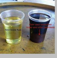
moisture which can corrode brake and clutch internal parts. A used container of hydraulic fluid can absorb moisture and should be discarded after initial opening. Also, using an incorrect fluid like DOT 4 when your system requires DOT 5, can cause rapid deterioration and failure of your system. And, finally, if your hydraulic system isn't serviced correctly, you may get air in it which will reduce the efficiency of your system.
