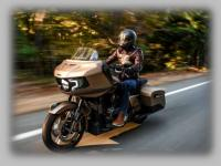
inch (1,768cc) mill produces a claimed 122 horsepower and 128 pound-feet of torque. Tied into a cast aluminum frame housing a big, fixed fairing, Challenger weighs 796 pounds dry.
