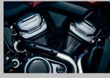
Minimizing weight and maximizing performance, the Revolution Max provides a powertrain narrow profile that is integrated into the motorcycle as a stressed member of the frame to enhance center of
