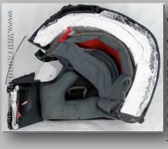
There is a comfort liner that riders often mistake for a protective component, which also does provide some padding. A helmet should also have EPS foam in the lower area to adequately protect the face and jaw.
