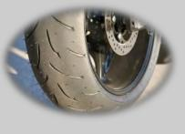
When storing on stands, reduce the tire pressure by 20 percent. If this is not an option, fill the tires up to their maximum recommended pressure and check the pressure every month. Periodically spinning the tires so that the bike's weight rests on different portions of the tread is also helpful.
