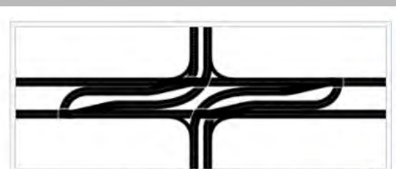
At a superstreet, all traffic on the side road must turn right, where it can access a U-turn ramp. Traffic on the main road can turn left directly. The opposite applies for countries that drive on the left.
