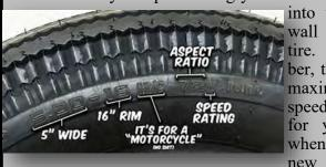
into the sidewall of each tire. Remember, this is the maximum speed rating for your tire when it was
