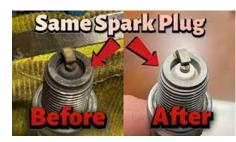
Prevent problems down the road by checking your motorcycle's **spark plugs**. If any are dirty or show signs of damage, replace them before you are left stranded on the side of the road.
