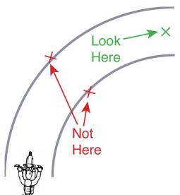
When a rider looks in a particular direction, their body naturally leans slightly in that direction, causing a very subtle counter steering input. This input, even if unconscious, can cause the motorcycle to lean in the desired direction. Additionally, the rider's focus on a specific point can influence their body's natural movements, contributing to the motorcycle's response to their gaze
