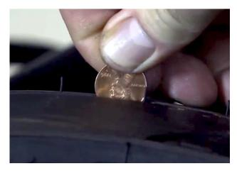
should be taken as close to the middle of the tire as possible. Your tire also has Tread Wear Indicators (TWI). You have little arrows placed around the tire on the sidewalls identifying the approximate TWI locations. If your tread is worn down to the TWI you need to replace your tire.
