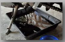
the bottom of the pan. It needs to be stirred up to ensure it escapes when you pull the drain plug. Starting the engine and letting it idle for a minute or two is perfect for that final circulation. Run it any longer and it does nothing more than than burn you. Before Be sure to have your oil drain pan you pull that drain plug, give the engine a minute after shutting down, allowing the oil to drain to the pan from the nooks and crannies in the engine.
