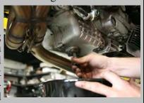
the plug by hand, push in–against the plug as it comes out—so the threads act as a seal with the outer edge. With a little practice you can get the pressure right and can spin the plug a full turn to feel for the "click." That click means the plug overlapped the last thread. With a swift motion away from the direction of oil flow, remove that now-loose plug. This can make warm, thin viscosity oil changes much cleaner and sometimes spotless.
